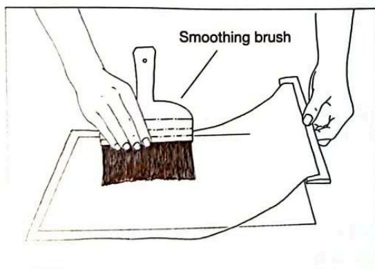
5. Lower the lifting bamboo slowly while using a smoothing brush to smooth the paper.
